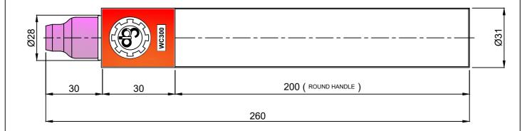
NOTE: 1) ALL DIMENSIONS ARE IN MM. 2) HEAD LENGTH WILL VARY AS PER LENGTH OF ARGON ARC NOZZLE
