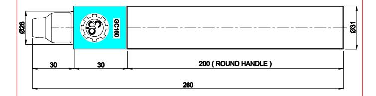
NOTE: 1) ALL DIMENSIONS ARE IN MM 2) HEAD LENGTH WILL VARY AS PER LENGTH OF ARGON ARC NOZZLE
